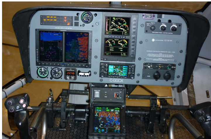
EC130B4 with Garmin G500H, GNS430W, GTS800, RA-4500 & Customer Specified Avionics Package including GTN750
