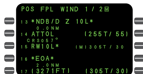
You can view and edit wind data for flight plan waypoints, increasing accuracy of position predictions and ETAs.
