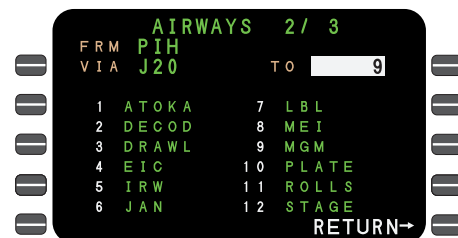
All the airway waypoints between your entry and exit will be automatically inserted into the flight plan.
