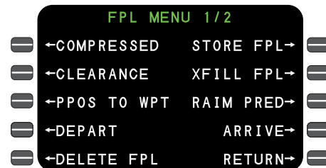
Menu format provides selections for flight plan displays, SIDs, STARs, approaches, flight plan storing and reversing.
