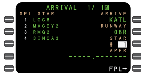
Select the runway, STAR and transition; the full procedures for the desired arrival will be added automatically to the flight plan.
