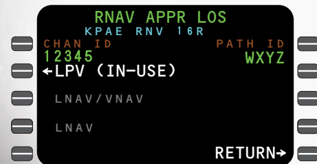
WAAS/SBAS-FMS Approach Mode provides ILS-like guidance with LPV, LNAV/VNAV and LNAV level of service for RNAV (GPS) approaches.
