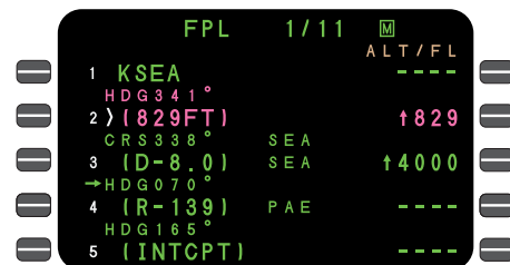
Normal view of flight plan pages shows a wealth of information including altitude restrictions.
