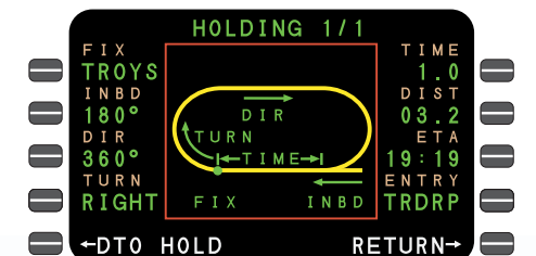
Holding patterns are accurately flown through the WAAS/SBAS-FMS automatically, complete with appropriate entry procedure: direct, parallel or teardrop.
