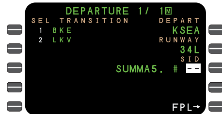
Select the runway, SID and transition; the full procedure for the desired departure will be added automatically to the flight plan.
