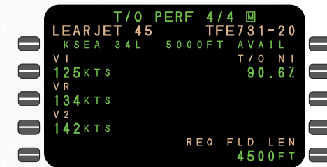
T/O speeds, runway length and N1 settings from AFM Performance Charts stored in memory.
