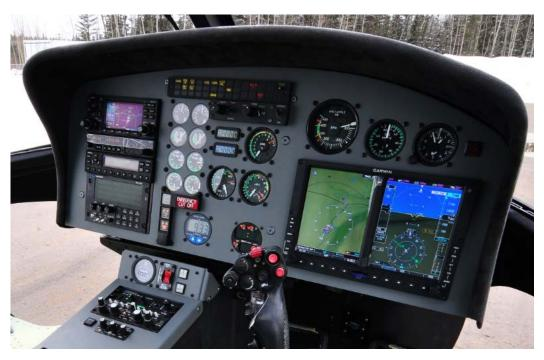
AS355N with Garmin G500H, GNS430W, GTS800, RA-4500 & Customer Specified Avionics Package
