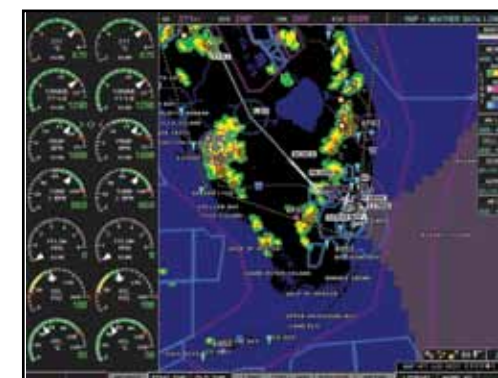
Weather datalink capability, via XM Satellite Radio and its XM WX Satellite Weather service, provides the G1000 with color NEXRAD, METARs, TAFs, lightning, and other U.S. data displays (subscription required).
