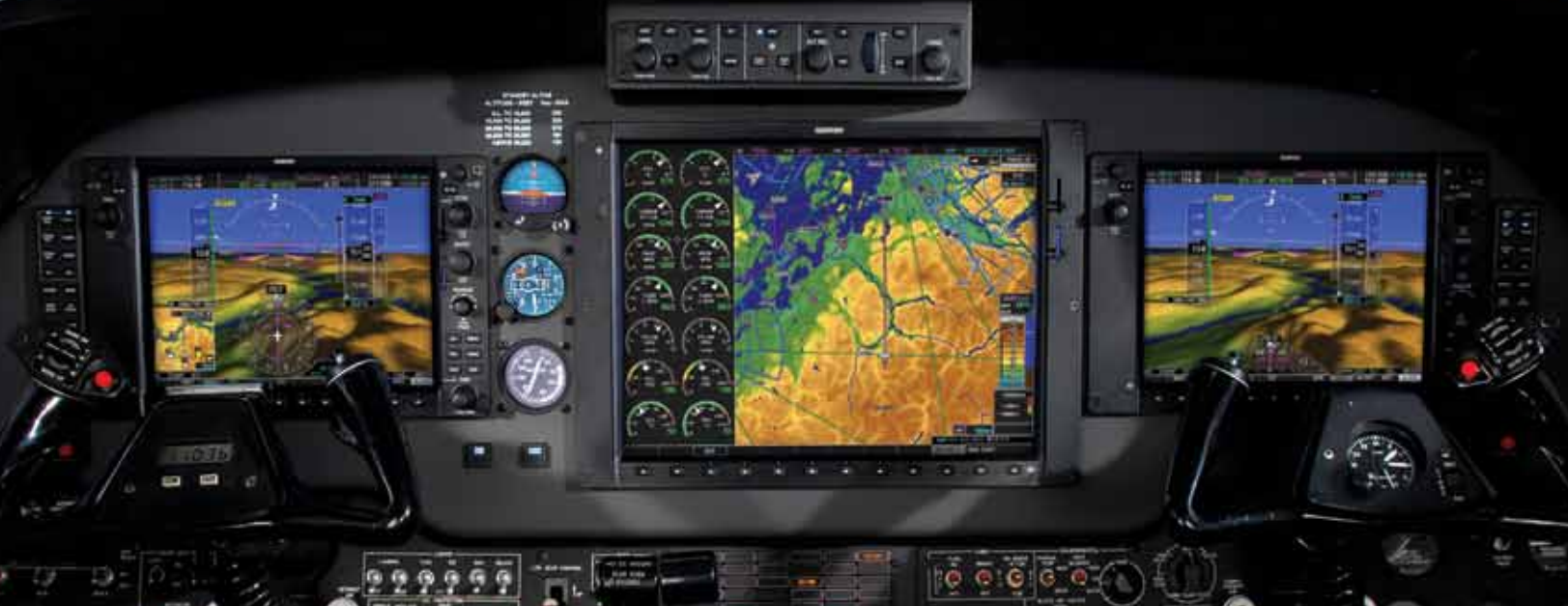
The King Air's 3-screen configuration features a big 15-inch Multi-Function Display (MFD) flanked by dual 10-inch Primary Flight Displays (PFDs). A Garmin autopilot mode controller, FMS keypad and dual audio panels complete the package.
