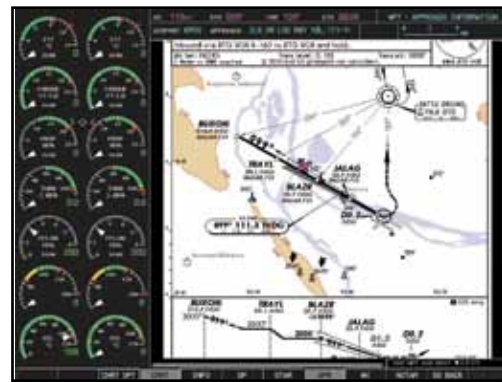
Optional ChartView™, powered by Jeppesen, lets pilots accurately overlay their aircraft's position on approach procedures and airport diagrams. Standard Instrument Departure and Arrival charts (SIDs and STARs) are also provided.
